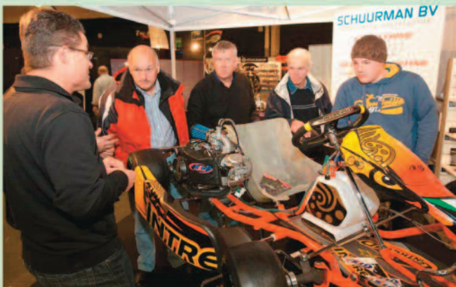
Schuurman BV showed off their 'made for karting' RK1 engine which has already proved popular in their native Holland and is set to be introduced in Belgium and Germany this year. The 150cc air-cooled 4-stroke has a built in generator and oil pump, a centrifugal dry clutch, electric start and produces 15hp. We hope to test this quiet, low maintenance and economically priced engine in the very near future Photo: Chris Walker
