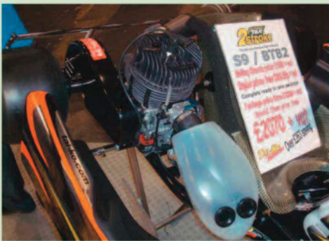
Tal-Ko had their new TKM S9 kart on display with 50mm axle. The S9 has a 104.5cm wheelbase while smaller drivers can opt for the S9S which has a 102cm wheelbase. The TKM TAG engine was reported to be selling well following its launch at the 2008 show.
