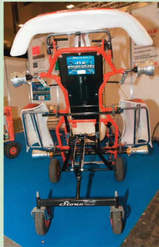
The Stone lift kart trolley imported by Karting4All is very handy for when no-one else is around
