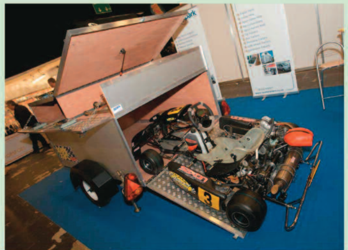
Spark Trailers & Towbars of Co. Durham have produced this bespoke trailer specifically for karters. The kart is stored in the lower section of the trailer while the top two sections can be used to store tools and spare parts. There is even a fold-out workbench Photo: Chris Walker
